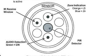
The sensor will dim the lights to 50% where the ambient light levels are very high
