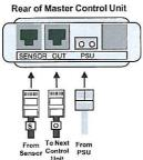
Sensor & Lamp Connections-Insert the cable into the sensor. Note the position of the jumper SW1 (for more information see section 10). Do not fit the sensor into the ceiling at this stage.
